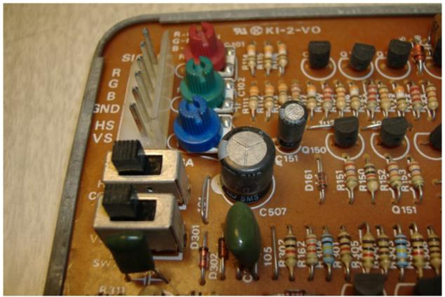
This monitor may be labeled as "KTA-915" or "T & E" or "KI-2-VO" or "JC-TRON" and sometimes might mistakenly be called a Samsung or Orion monitor depending on what brand of picture tube is installed on the chassis. Look on the foil (solder) side of the main monitor board (this assumes you have it already out and laying in front of you) for "KT-1420A" silkscreened near the edge of the board frame by transistors Q101 and Q102.
